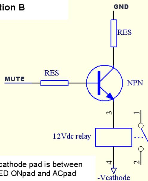
Option B shows the circuit with a relay output. The relay can have more than the one set of contacts shown on the schematic which make it possible to control either signal input or output of the amplifiers.
