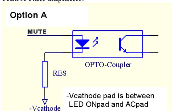
Option A shows the simplest way to control a low power enable control input of the amplifier module. The transistor output might have to be a Darlington coupling and/or have to have a series resistor.
